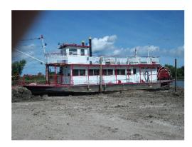
To get it there we built a levee around the boat and pumped water into the pond and floated it over onto the blocks. Then broke the levee letting the water go out. Total cost \$100 bucks for fuel. I own the dozer, excavator, and water pump only took 3 hours.
